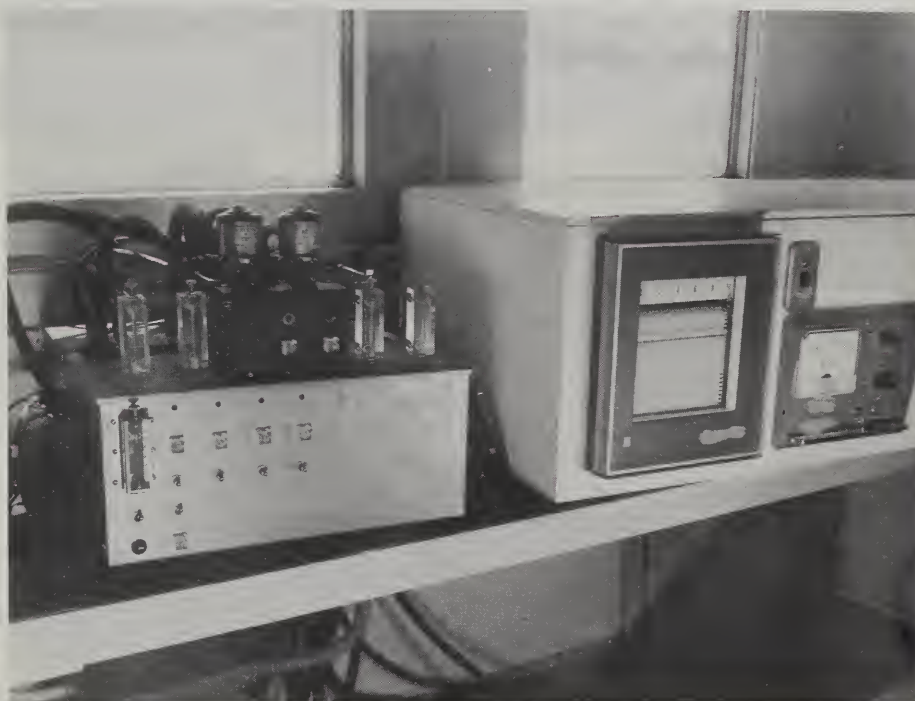
Figure 5.--Carbon dioxide control instruments. Shown, from left to right, are the station selector (constructed by project personnel), carbon dioxide induction valve (constructed by project personnel), recorder controller (Honeywell Elektronik 17, 0 - 100 mv), and infrared gas analyzer (Mine Safety Appliances, Lira Model 300, 0 - 2000 ppm carbon dioxide in air).
